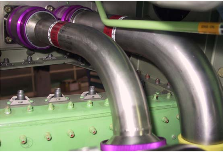
Stainless Steel Wolfbend™ Fuel Lines in Engine Pylon
